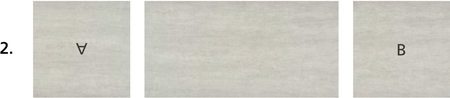
Rotate part A 180° and join parts A & B to the full slab
