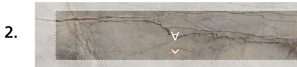
Rotate part A 180°. Plan to join parts A & B for continuation of the main vein and remove the surplus.
