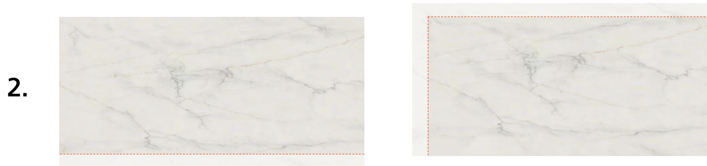
Plan to join the two slabs for continuation of the main veins and remove the surplus
