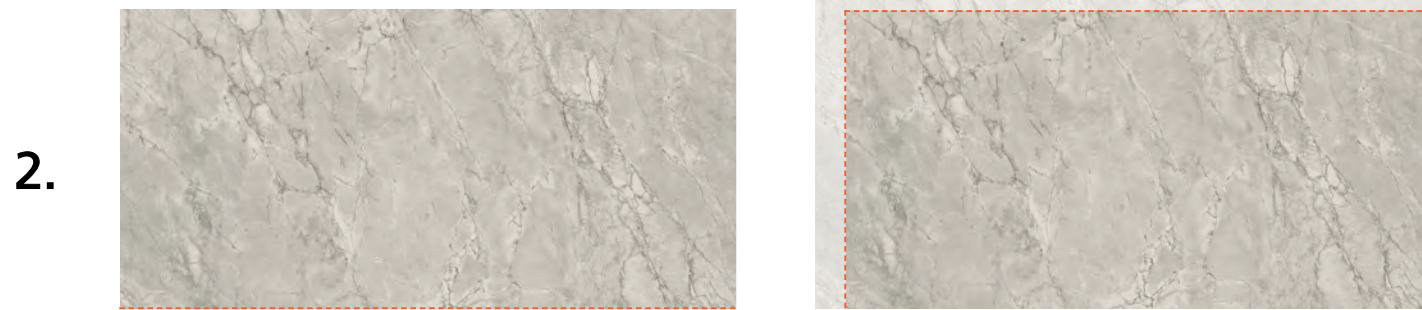
Plan to join the two slabs for pattern continuity and remove the surplus
